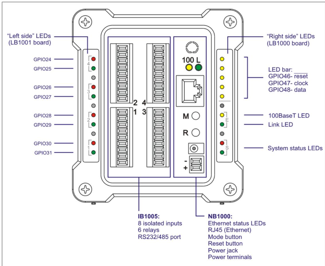
The DS1005 BASIC-programmable controller features eight opto-isolated digital inputs, six high-power relays, and one RS232/485 port.
