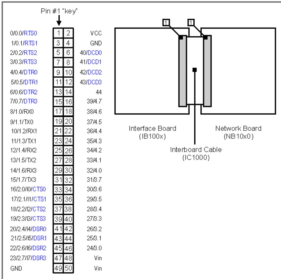
*Note 1: indicated pin functions correspond to the pin functions of the [EM1000](#) module (installed on the [NB10x0](#) board). To save space, "GPIO" and "P" were omitted. For example, "17/2.1" actually means "GPIO17/P2.1". "I1" means "INT1".*
