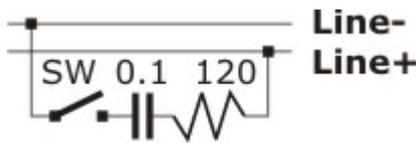
If you are using RS485 mode (SW1 and SW2 are closed) and you want to terminate the RS485 bus, then you only need to close either SW5 or SW6. Having both switches closed will effectively add two termination circuits to the same bus!
