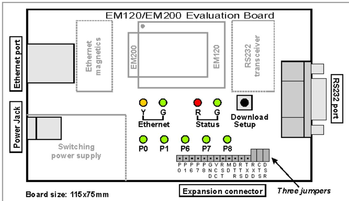
The EM120/200-EV Evaluation Board offers a convenient way of testing the [EM120](#) and [EM200](#) embedded modules. The board features the following components:
