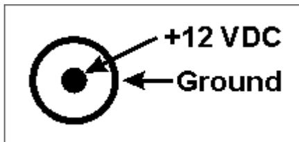
Alternatively, you can power the board through the Vin line on the [expansion connector](#). Two onboard diodes combine power jack and Vin inputs into a single line, which goes to the switching regulator. Clean 3.3V output produced by the regulator is used to power the EM1206EV board itself, the [EM1206](#) module, and optionally an add-on board plugged into the [wireless add-on connector](#). This 3.3V power is available on the expansion connector as well.
