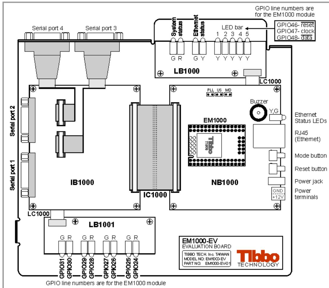
The EM1000-EV Evaluation System offers a convenient way of testing the [EM1000](#) BASIC-programmable embedded module. The board features the following components:
