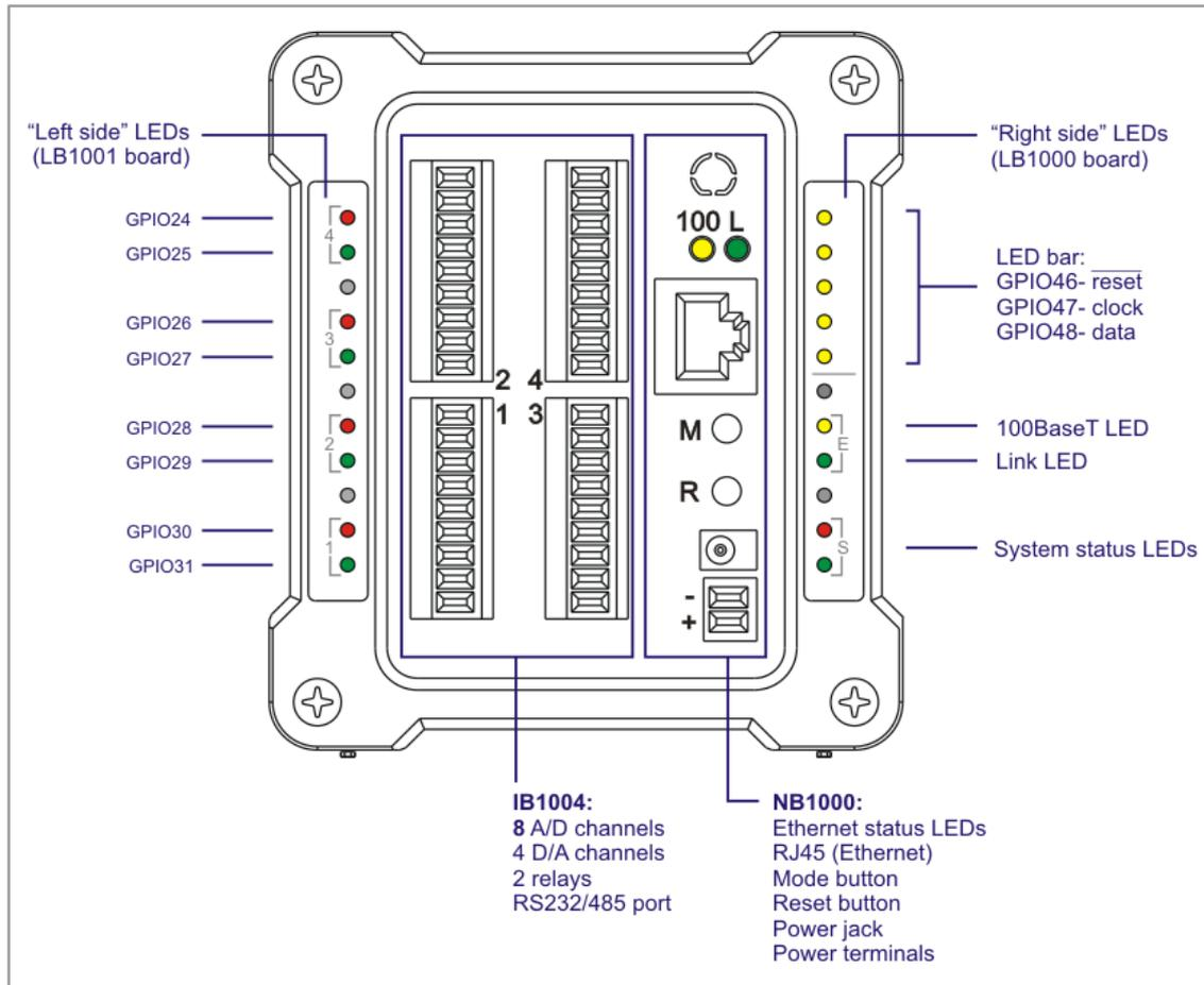
The DS1004 BASIC-programmable controller features eight A/D inputs, four D/A outputs with both voltage and current outputs, two low-power relays, and one RS232/485 port.
