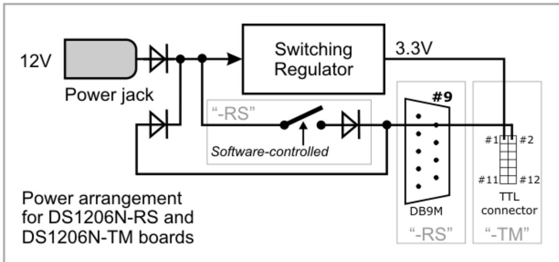
Tibbo serial-over-IP application supplied with the DS1206N has a dedicated "PS" ("Power on pin 9") setting to control the power switch. To turn the power switch on from within your Tibbo BASIC application, enable (configure as output) line PL\_IO\_NUM8\_PWROUT and then set this line to HIGH. Additional programming information can be found in "TIDE and Tibbo BASIC Manual" (see i.o object and DS1206 platform documentation).
