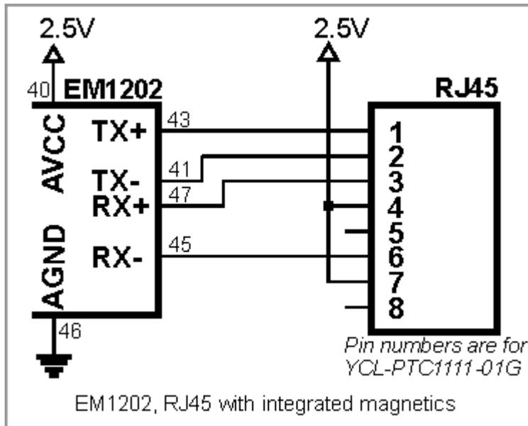
It is important to make the PCB wire connections between the Ethernet port pins of the EM1202 and external magnetics circuitry as short as possible. Making the wires too long may cause the noise level generated by your PCB to surpass the maximum radiated emission limits stipulated by FCC/CE regulations. Additionally, longer Ethernet lines on the PCB will make your board more susceptible to the damage from the ESD (electrostatic discharge). Follow these three recommendations:
