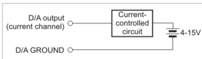
The D/A converter has full galvanic isolation from the rest of the IB1004 + SB1004 circuitry: the power for the D/A section is generated by an isolated switching power supply, all control lines use opto-couplers.
