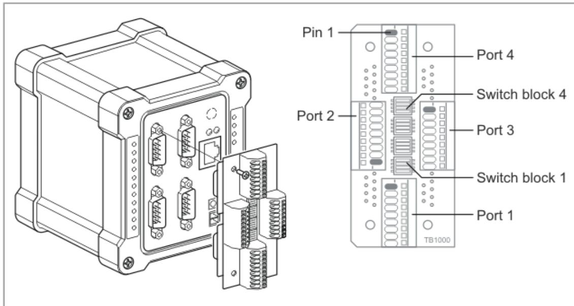
The TB1000 terminal block adaptor mounts on [DS1000](#), [DS1002](#), and [DS1003](#) devices (or [IB1000](#), [IB1002](#), and [IB1003](#) boards). This adaptor "converts" DB9 connectors of the DS1000, DS1002, and DS1003 into 9-terminal blocks of "spring clamp" type. These are convenient for attaching wires, which is very useful for industrial installations.
