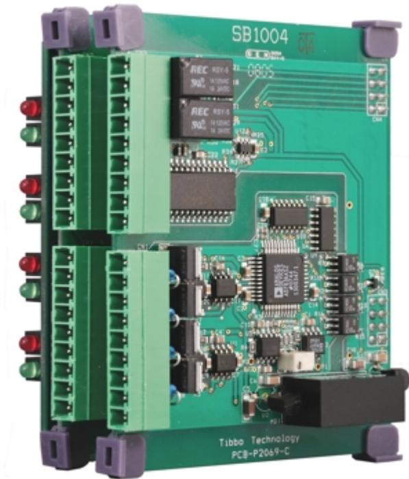
The IB1004 is the main board in the pair, and is connected to an [NB10x0](#) network board by the [IB1000](#) interboard cable. The SB1004 is a supplementary board, it exists because a single IB1004 would not be able to accommodate all required circuitry and terminal blocks. In the board pair, the IB1004 carries the A/D converter, while the SB1004 contains the D/A converter, RS232/485 port, and 2 low-power relays.
