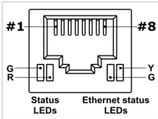
Ethernet port of the EM1202EV is of 10/100BaseT type. Connector is of RJ45 type, pin assignment is as follows:
