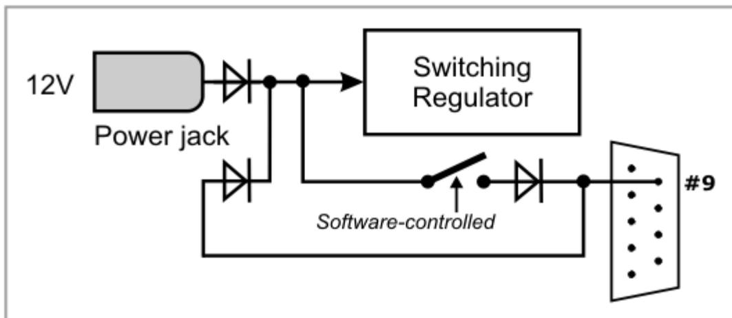
Tibbo serial-over-IP application supplied with the DS1206 has a dedicated "PS" ("Power on pin 9") setting to control the power switch. To turn the power switch on from within your Tibbo BASIC application, enable (configure as output) line `PL_IO_NUM8_PWROUT` and then set this line to HIGH. Additional programming information can be found in "TIDE and Tibbo BASIC Manual" (see i.o object and DS1206 platform documentation).
