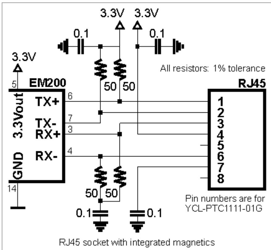
It is important to make the PCB traces connecting the Ethernet port pins of the EM200 to the magnetics circuitry as short as possible. Making the wires too long may cause the noise level generated by your PCB to surpass the maximum radiated emission limits stipulated by the FCC and CE regulations. Additionally, longer Ethernet lines on the PCB will make your board more susceptible to the ESD (electrostatic discharge) damage.
