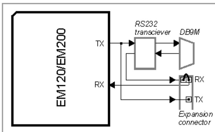
Maximum load for all CMOS-type lines (P0, P1, ... RX, TX...) is 10mA.
