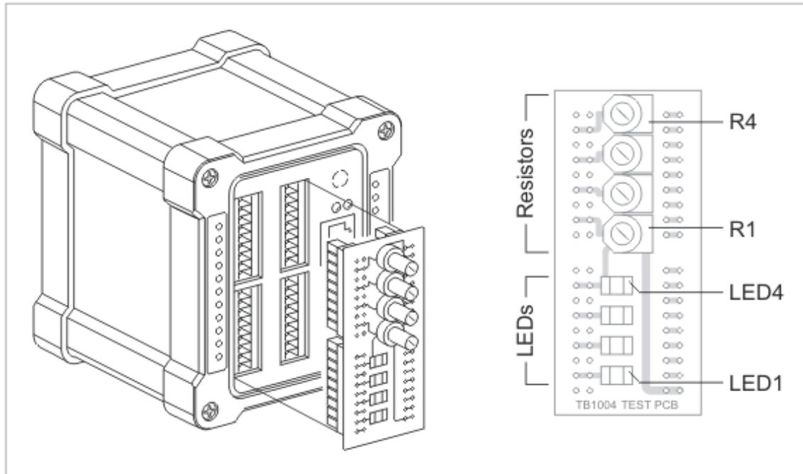
The TB1004 test board is provided for the convenience of evaluating the [DS1004](#) controller ([IB1004](#) + [SB1004](#) boards). The board is basically a loopback, feeding D/
