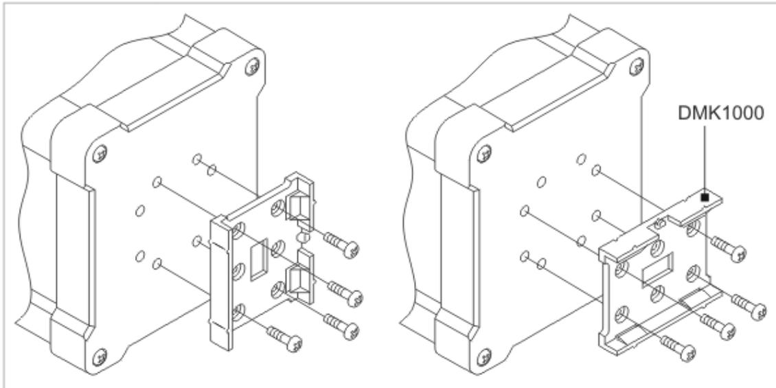
All DS10xx devices are supplied with the DMK1000 DIN rail mounting kit. Mounting holes on the back of the device allow you to attach the DIN rail mounting bracket horizontally or vertically.
