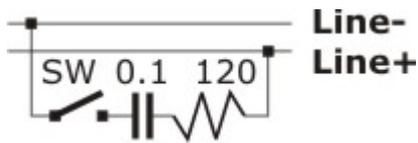
Notice, that if you are using RS485 half-duplex mode (SW1 and SW2 are closed) and you want to terminate the RS485 bus, then you only need to close either SW5 or SW6. Having both switches closed will effectively add two termination circuits to the bus!
