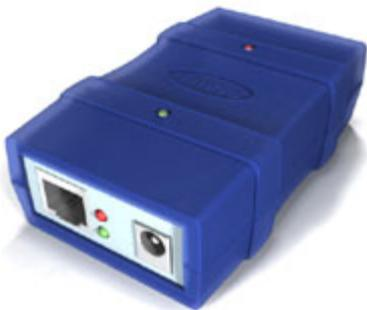
The DS100 is a Serial Device Server for external use. Device hardware includes one 10BaseT Ethernet port, one serial port and an internal processor that "glues" network and serial sides together. Internally, the DS100 is based on the [EM100 Ethernet Module](#).
