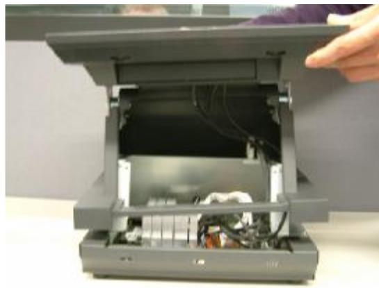
d. Lift the stand cover up to separate it from the stand base
