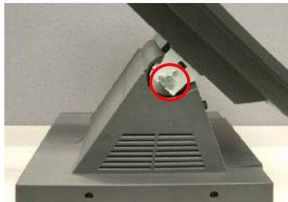
b. Remove the screws(6), 3 from each side to separate the display from the stand
