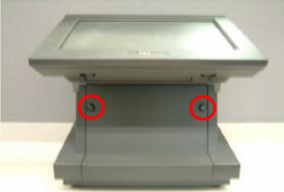
a. Loosen the thumb screws (2) to remove the front side stand cover.
