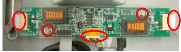
d. Remove the screws (2) and disconnect the cables (3).
