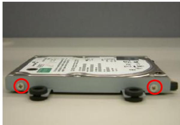
d. Remove the screws(4) (two from each side) to release the HDD holders(2) from the HDD
