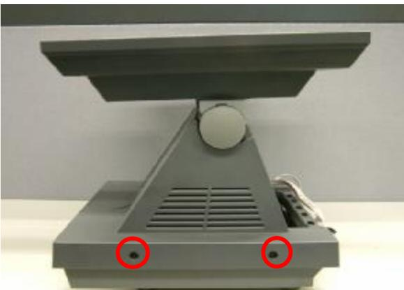
c. Remove the screw (4), 2 on each side, from the base
