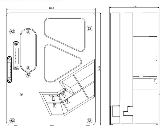
Figure 6: Overall dimensions (mm)
