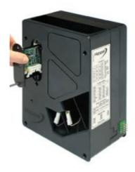
Figure 4: PCB removal
