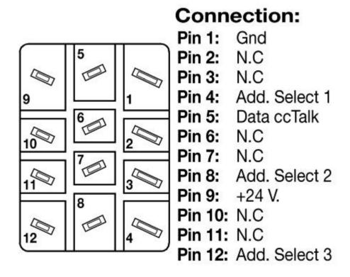
**pin 1** is the ground line and **pin 9** is the power line.
